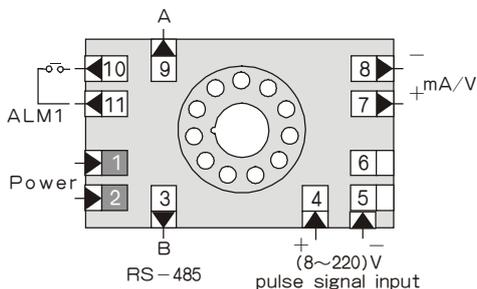
>> **Wiring diagram for WP 202 series isolation transformation module**
