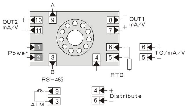
>> **Wiring diagram for WP201 series intelligent frequency transformational module**
